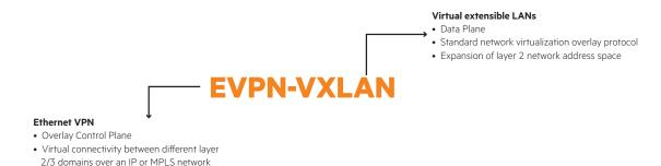
Figure 3. EVPN/VXLAN standards-based overlay fabric
